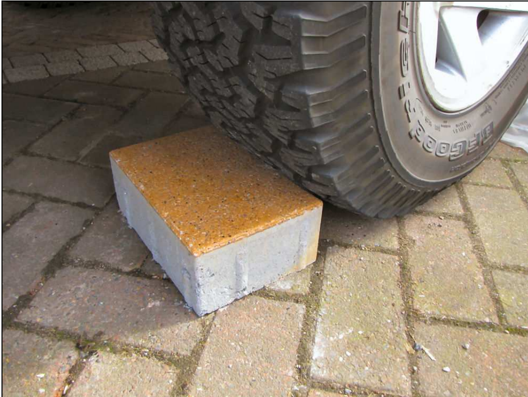
Figure 9 - Trafficking test on 80mm Trento Block Paver
