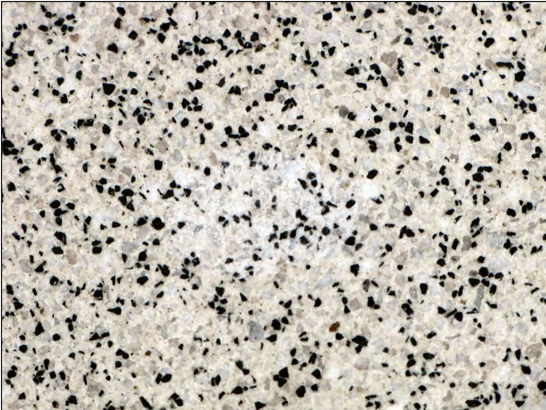
Figure 14 - A faint lightening of the surface where it has been in contact with paint stripper for 3 days
