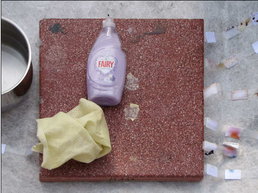
Figure 5 - Initial cleaning with warm water and detergent Note how label strips have had to be peeled off and placed to one side
