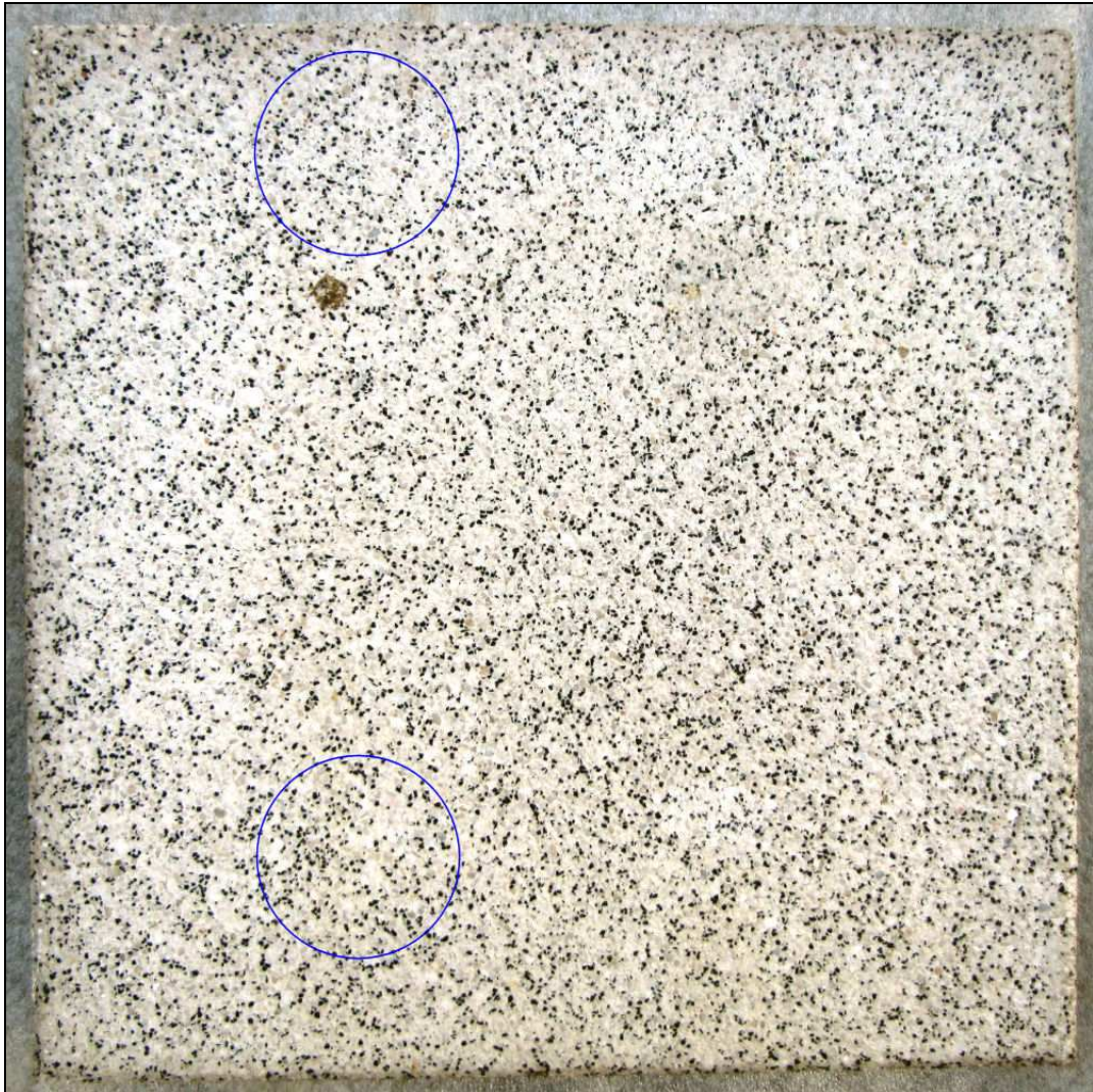
Figure 13 - Stains completely removed Other marks visible in this image arise for subsequent testing on this flagstone
